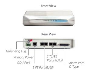
The 19" rack mountable IDU for Intrepid and Intrepid Ultra provides 2 FE ports and up to 8 T1/E1 ports (4 T1/E1 shown).
