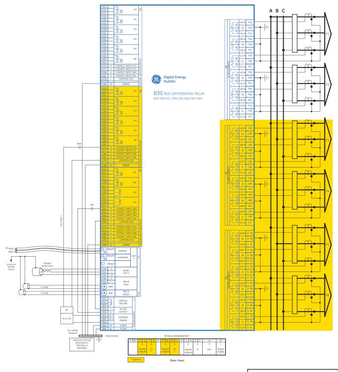
NOTE: This diagram is based on the following order code: B30-H00-HCL-F8H-H6H-L8H-N6A-S8H-U6H
