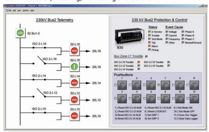
The B30 is the single point for protection, control, metering, and monitoring in one integrated device that can easily be connected directly into DCS or SCADA monitoring and control systems like Viewpoint Monitoring.
