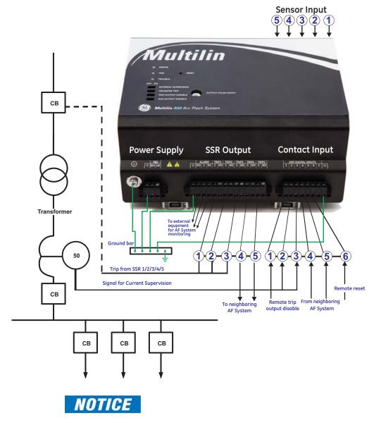
AFS device must be installed in an electrical enclosure with authorized access.
