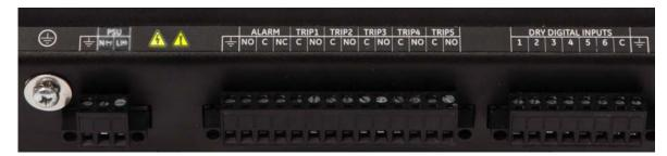
Figure 6: A60 Sensor connections
