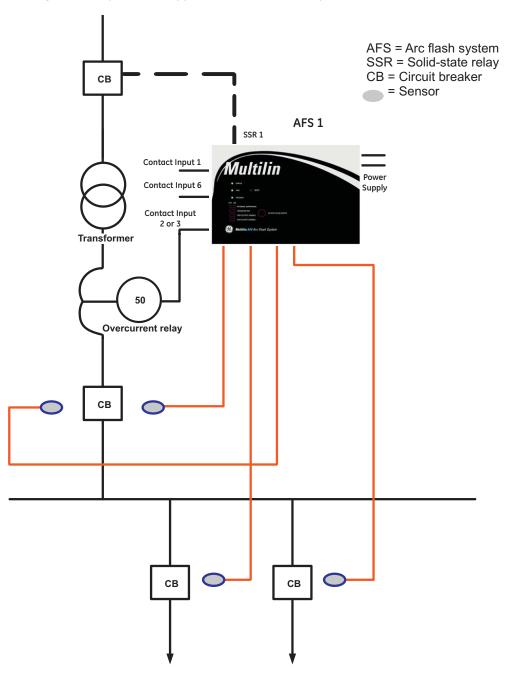
Figure 2: AFS protection application with current supervision enabled
